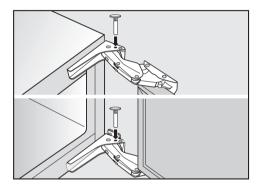
■ Place the locking pins supplied for limiting the door opening into the hinges from above.
